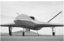
A new, reduced-signature, unmanned aircraft—the long-rumored, 20-hr.-endurance, pure-jet Predator C Avenger—has emerged from General Atomics Aeronautical Systems' workshops after a 3½-year gestation period paced by massive growth in UAV production and the use of unmanned designs in combat.
